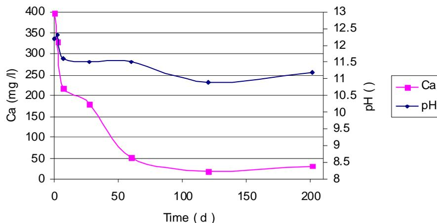
*Figure 8: Change in the pH and in the calcium concentration of the materials treated with 2.5% of lime on the Czech Republic site.*
