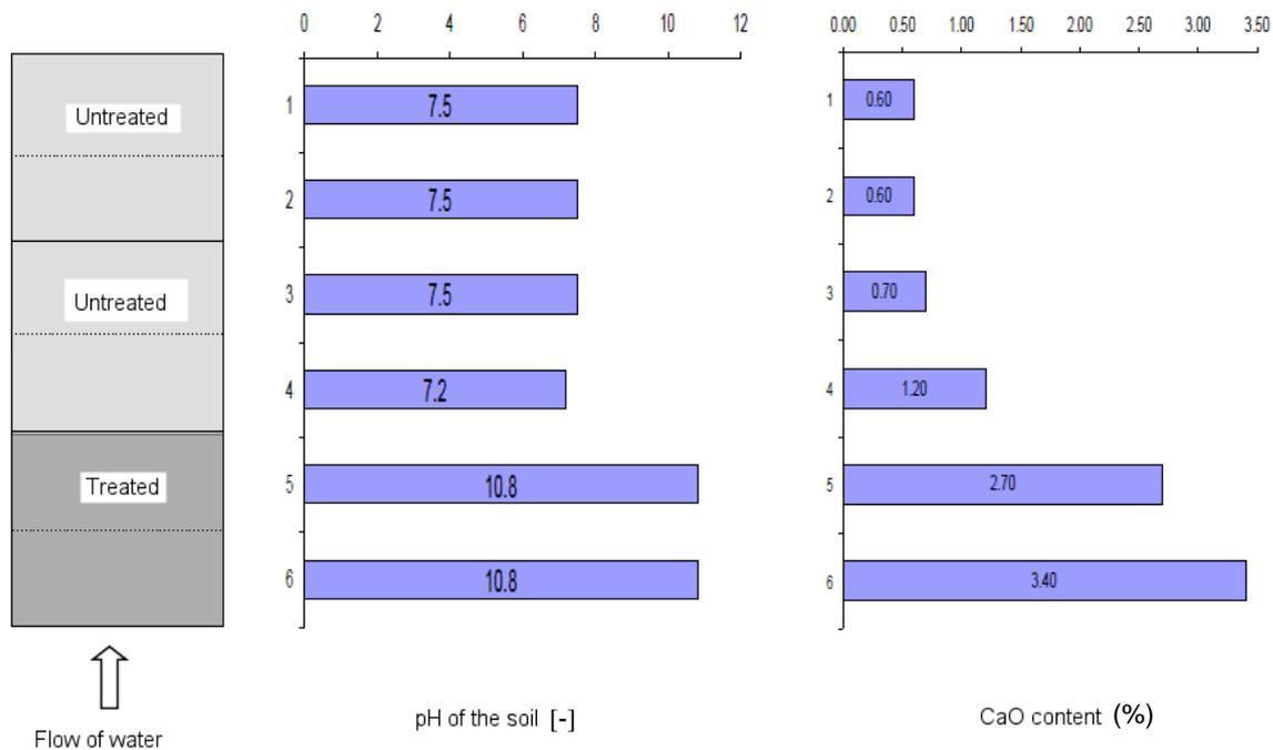
Figure 5: pH values of the different layers and total CaO content of the sample of silty soil treated with 3% of lime and untreated “buffer” soil, on conclusion of the percolation test.
