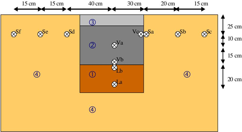
Figure 7: Scheme for withdrawing the samples from the experimental trench.
