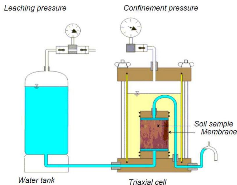
Figure 1. Experimental assembly of the leaching cell.
