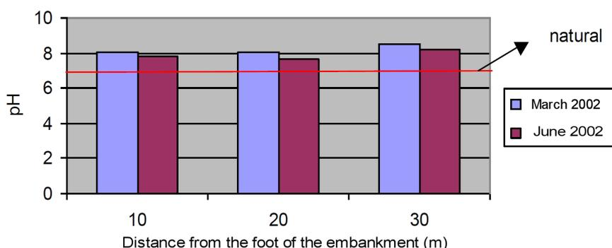
Figure 9: pH values measured in the water on conclusion of core borings at several distances from the soil body treated with 2.5% of lime.
