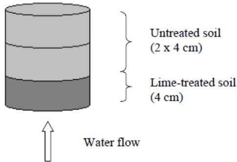
Figure 2. Arrangement of the soil sample subjected to the leaching test.
