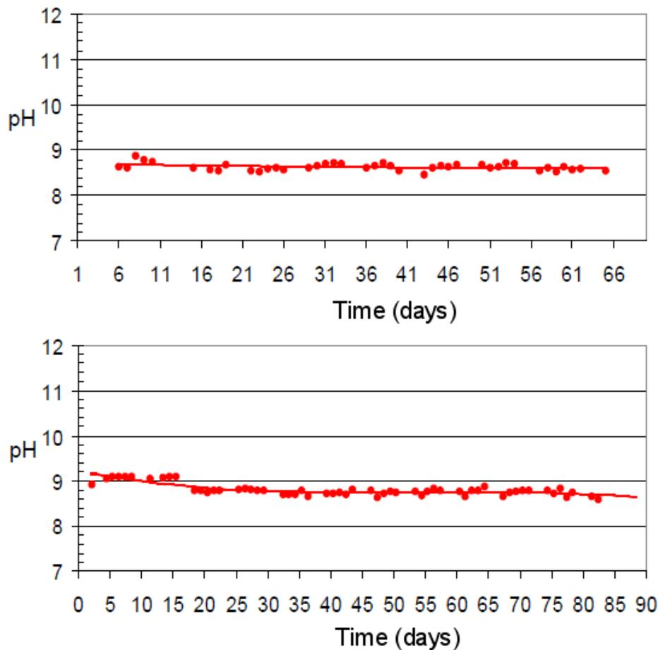
Figure 3. pH values of the leaching waters from the samples containing the silty soil treated with 1% (upper graph) and 3% (lower graph) of quicklime.
