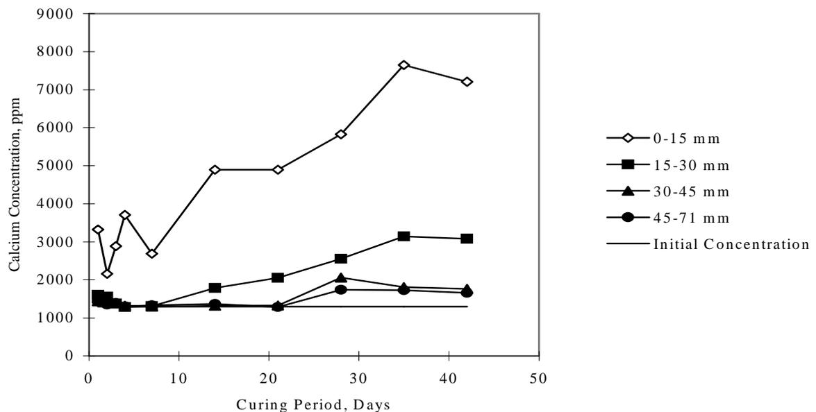
Figure 10. Relationship between calcium concentration in clay surrounding the lime pile, and curing period.
