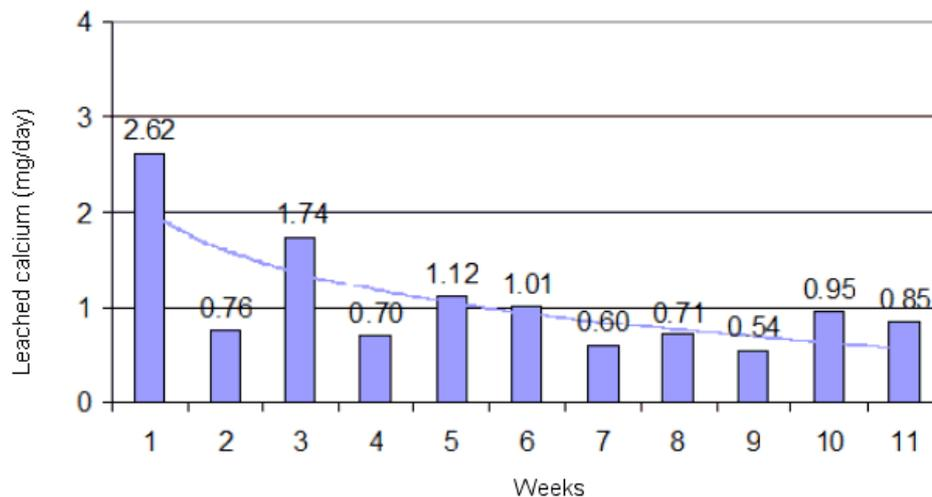
*Figure 4: Amount of leached calcium as a function of the time, from the sample containing the silty soil treated with 3% of lime.*
